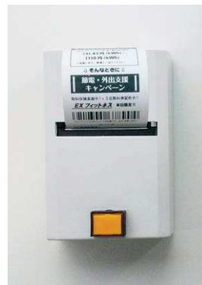
Fig.1 The HEMS Printer
